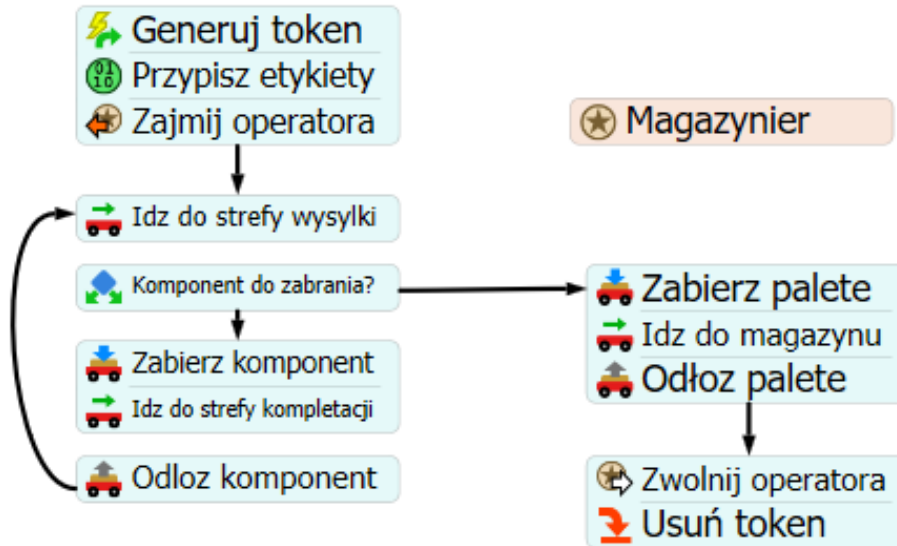
Fig. 24 Process Flow – tasks until the components are placed in the picking zone
